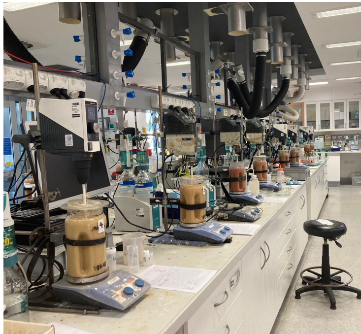
Figure 2: Diagnostic leach tests being conducted in the ANSTO Minerals Leach Laboratory, Sydney, NSW.
