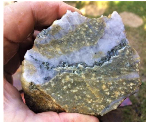
Johnston's Hill quartz vein with pyrite-galena-gold in intensely silica-sericite altered porphyry
