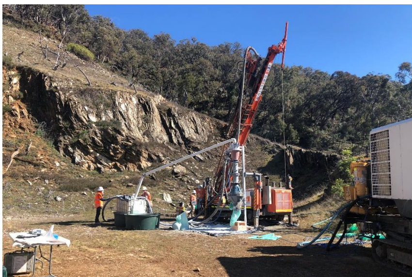
Figure 1: RC drill rig located on the first hole of the Quarry Lode drill program at Lewis Ponds. Drill rig is located in the old limestone quarry, which was active during the late 1800’s. Limestone was used as a flux in the historic Lewis Ponds smelter. Photo taken by J. Owens on 20 August 2021.
