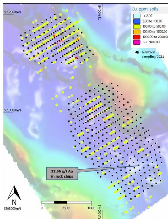
**Figure 2. A: Copper in soils results and infill soil program plotted on 1994 aerial magnetic survey TMI RPT, with location of high grade, 12.65 g/t Au rock chip noted.**
