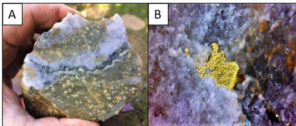
Figure 4: A - Johnston's Hill quartz vein with pyrite-galena-gold in intensely silica-sericite altered porphyry. B - Visible gold in hand sample from the Emu Prospect, in Gundagai North.
