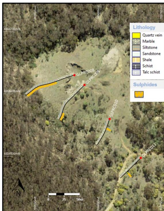
Figure 1. Plotted drill traces from the Quarry Lode drilling program at Lewis Ponds.
