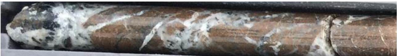
Image 1: Albite-chlorite-sericite-hematite altered micro-monzonite porphyry with crustiform banded quartz-carbonate chlorite with minor bornite and chalcopyrite from 471.4m in drill hole CHERCD013
