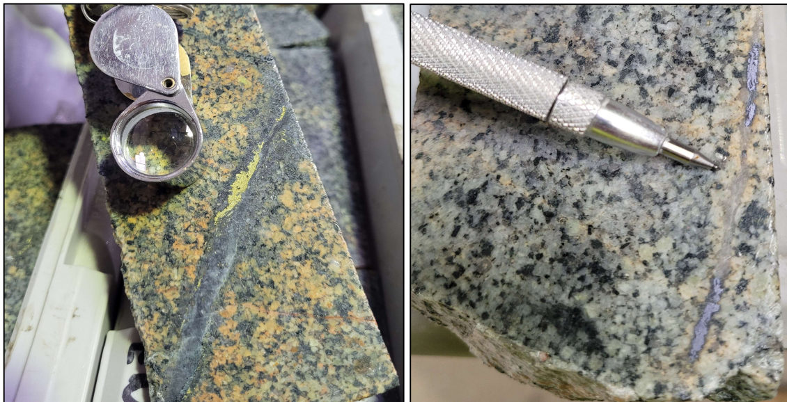
Figure 3: Vein hosted chalcopyrite (left) and molybdenum (right) mineralisation with albite-sericite-chlorite vein halo alteration in GYDD002.
