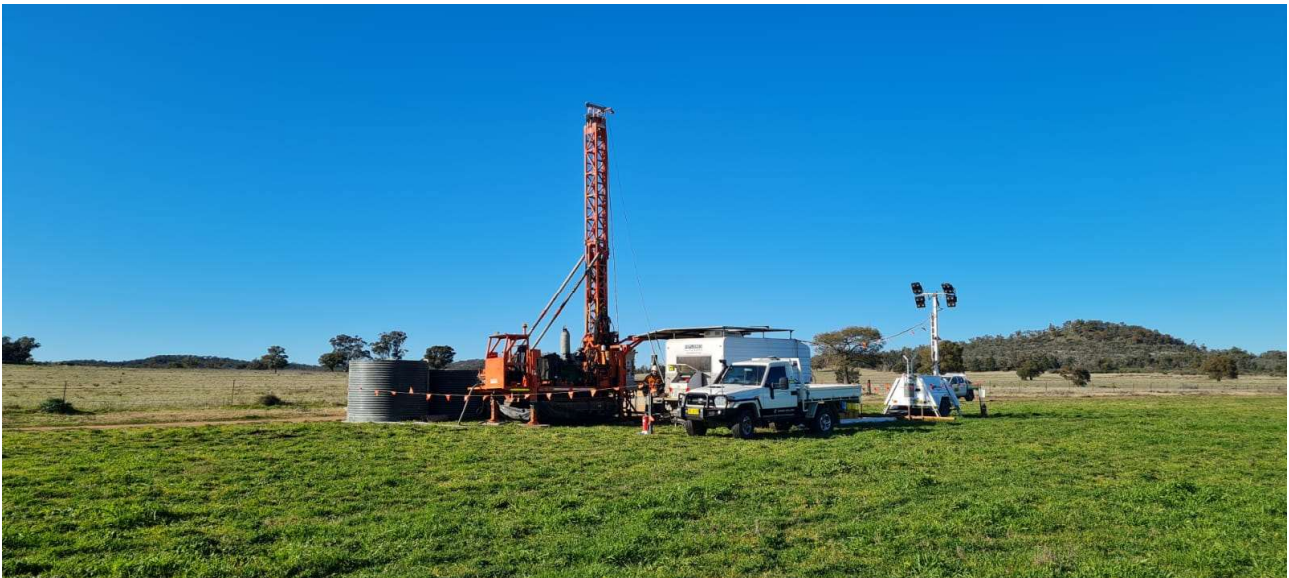
Image one: Diamond drill rig on site at the Narraburra Rare Earth Project
