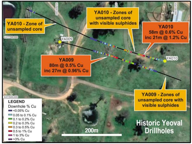
Figure 2: Location of YA009 and YA010 drill holes at the Yeoval Prospect. Copper values shown downhole in ppm
