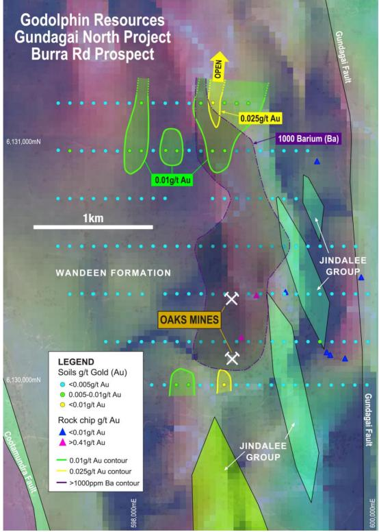
Figure 5: Burra Road Prospect soil and rock chip results with gold and barium contours. Seamless geology and NSW state-wide TMI imagery underlain
