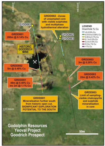
Figure 3: Plan view showing location of GRD001, GRD002 and GRD003 drill holes at the Goodrich Prospect
