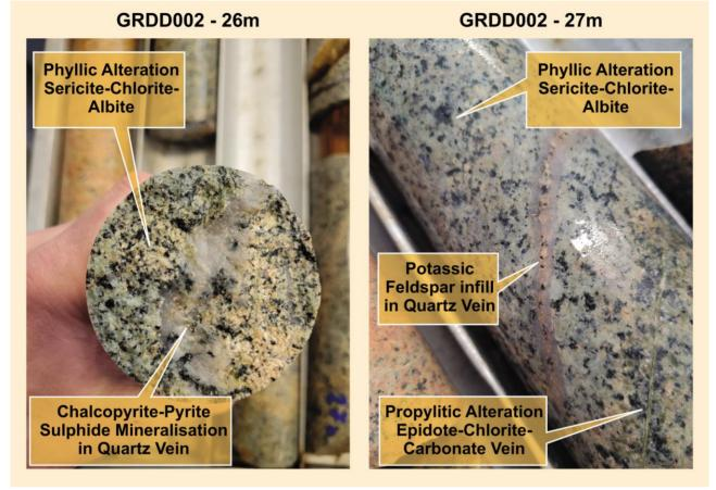
Figure 4: Photos of drill core from GRD002 showing A: quartz vein mineralisation, visual estimate of 0.2% copper mineralisation and B: multiphase alteration styles in unsampled core
