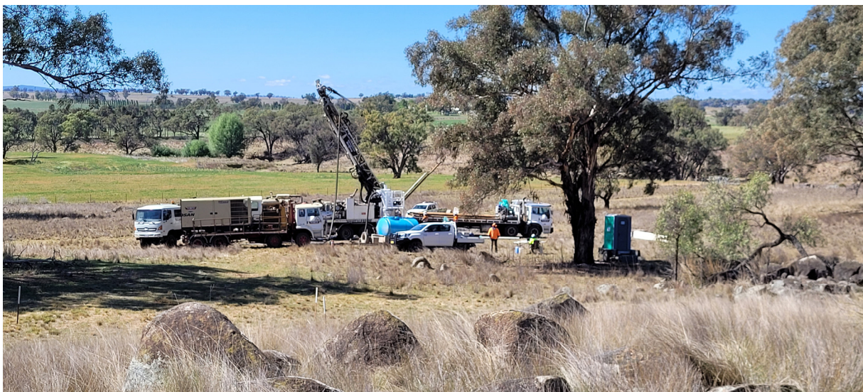
Figure 1: Drill rig at drill hole GYVRC001 – photos are looking generally northeast with drill hole inclined at 60 degrees to 220 degrees (True North). Note old workings on lode material on right hand side.
