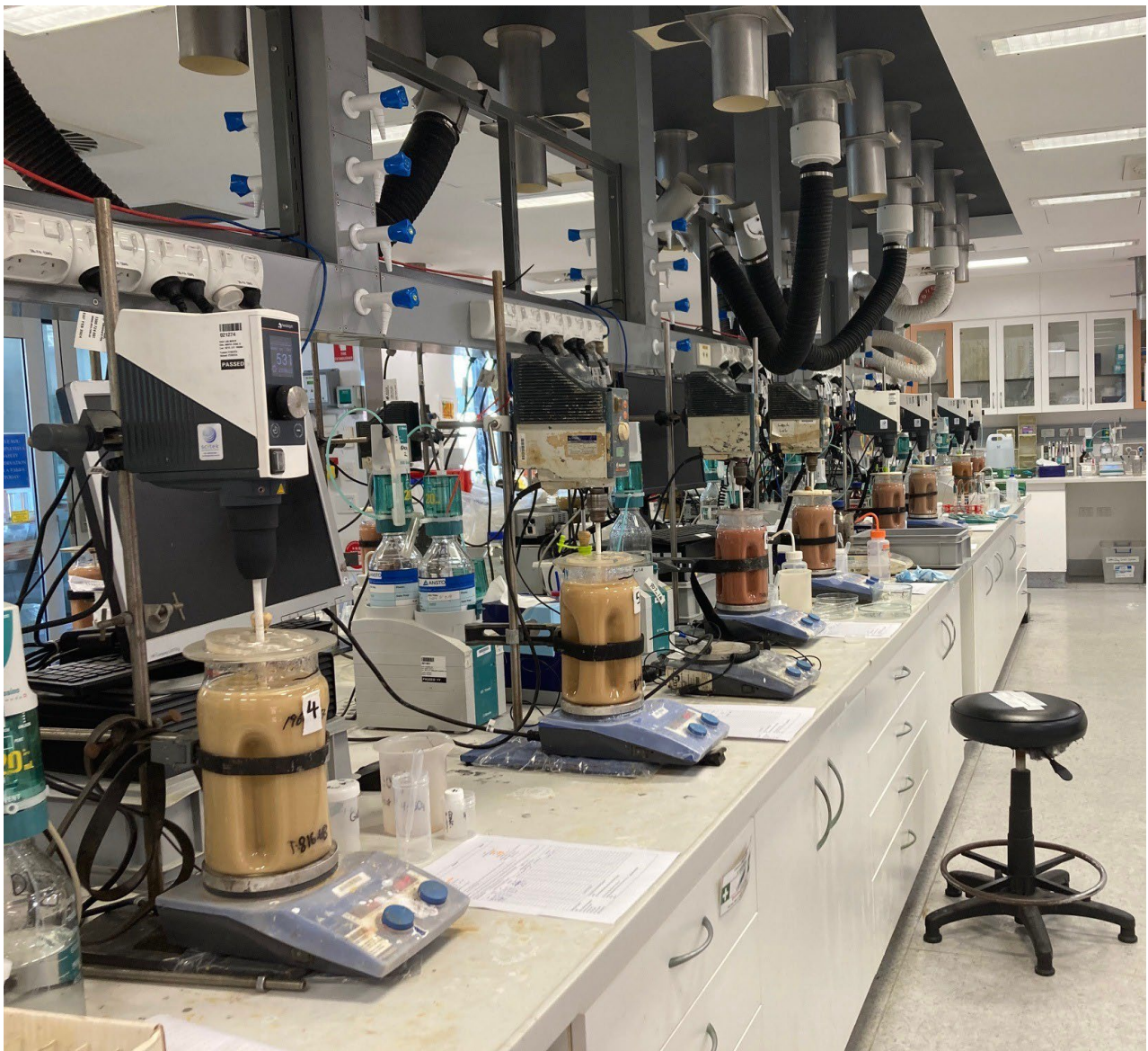
Figure 1: Diagnostic leach tests being conducted in the ANSTO Minerals Leach Laboratory, Sydney, NSW.
