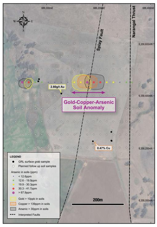
Figure 2: Spring Creek prospect showing the soil sample orientation line (displaying arsenic) and the gold-copperarsenic soil anomaly. A detailed soil survey has commenced to the north and south of the orientation line and along the Narangal Thrust splay fault (white circles).
