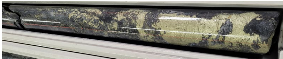
Vein hosted Chalcopyrite (Copper) magnetite and chlorite mineralisation from GYDD001 –
