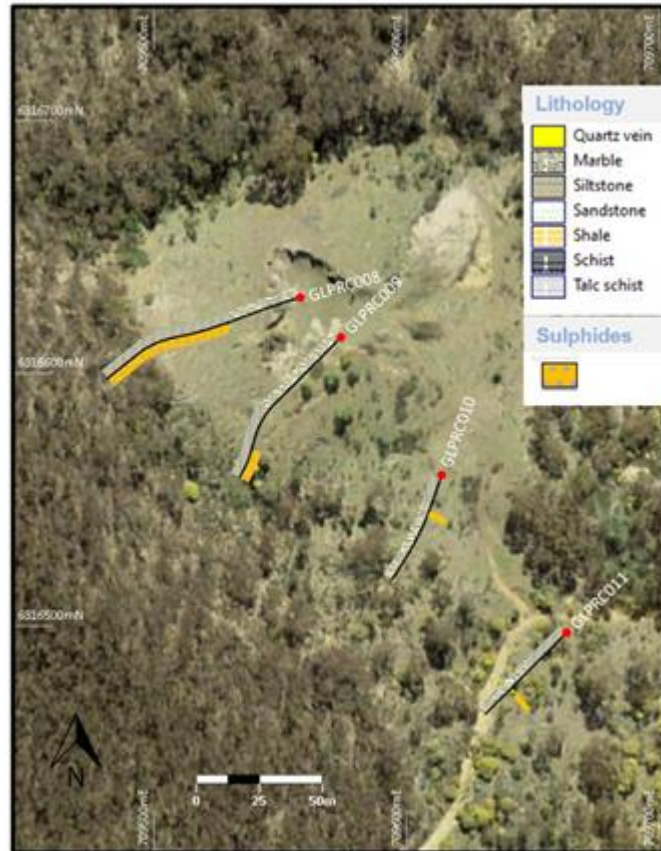
Figure 3: Plotted drill traces from the Quarry Lode drilling program at Lewis Ponds
