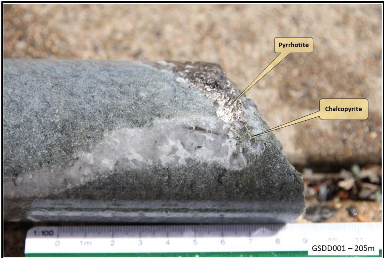
Figure 3: Quartz vein-hosted pyrrhotite and chalcopyrite mineralisation surrounded by chlorite-sericite altered arenite, 205m, GSDD001
