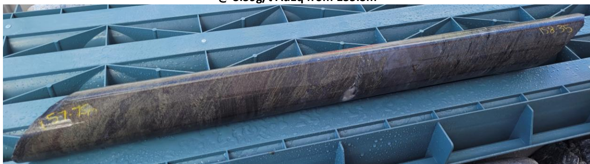
Figure 7: Photo of diamond drill core from GLPDD007 showing massive sulphide mineralisation grading into semi-massive sulphides with pyrite (yellow) and sphalerite (red) with galena and chalcocopyrite. Associated sample interval GRD11022 (157.6-158.15m) returned 13.69g/t AuEq
